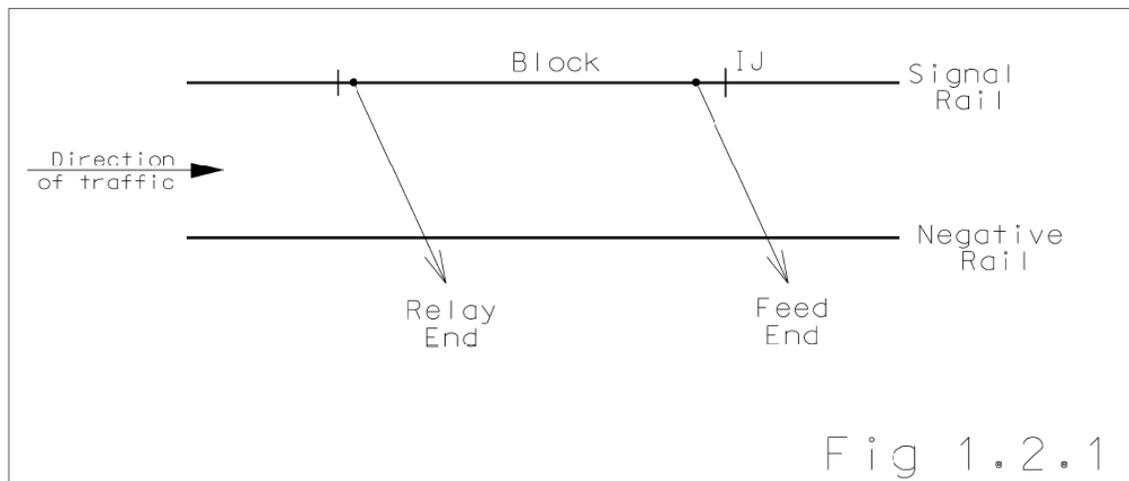
Figure 1.2.1: Single Rail Track Circuit
